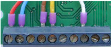
The bus connection section can be found after dismantling the connection section and removing the two screws on the printed circuit. The designation **A-Line** and **B-Line** is provided twice; this indicates, that the **PROFIBUS** is **looped internally**. Corresponding terminals to that purpose are already provided on the printed circuit. If the encoder is the **last member on the bus**, the bus termination must be activated.
