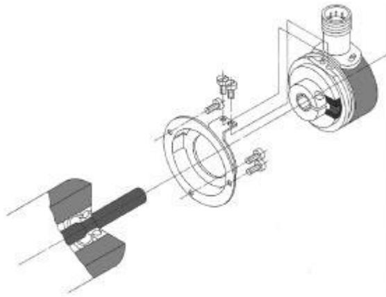
**Mounting with an assembly bell+coupling (Mainly shaft encoders)**
