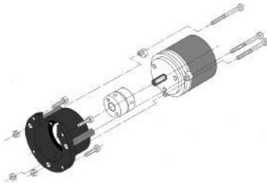
**Mounting with a bearing box (Shaft encoders)**
