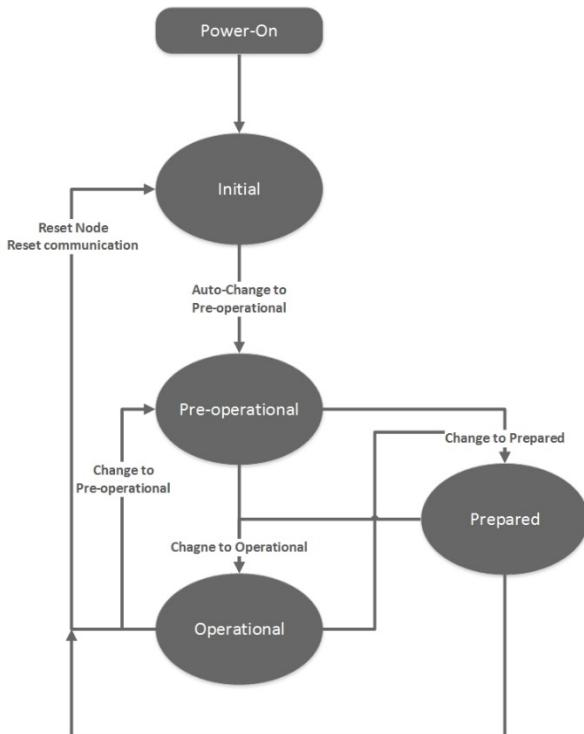
**Initialization:** this is the initial state after the power supply is applied, following a device Reset or Power ON. After performing the reset/initialization routines, the node switches automatically to the Pre-operational status. The LEDs display the momentary status.
