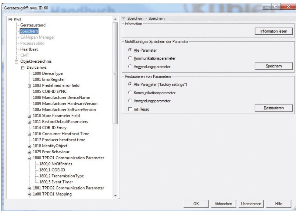
Switch then over to Operational Mode. The mapped objects of TPDO1 are sent in a 100ms cycle:
