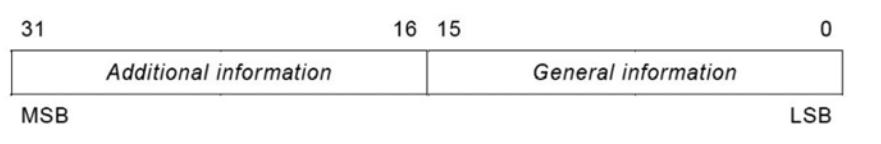
Bits 0-15      indicate the device profile version
