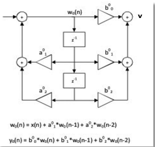
$X_n$  is here the input signal,  $Y_n$  is the **filter output and simultaneously the input** of another subsystem.
