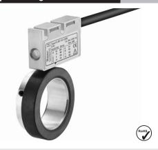
Thanks to its installation depth of only 16 mm, the bearingless magnetic rotary encoder RI50 / Limes LI50, comprising a magnetic ring and sensor head, is ideally suited for plants and machinery where space is very tight. The non-contact measuring principle allows for error-free use even under harsh environmental conditions, as well as ensuring a long service life. In contrast to our measuring system RI20 / Limes LI20, a single zero pulse is also implemented here.
