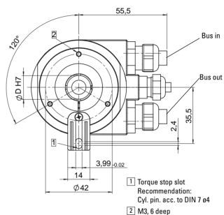
Blind hollow shaft version Flat bracket with double-win-
