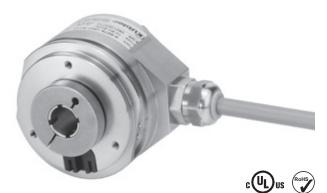
Thanks to their stainless-steel housing, the incremental hollow shaft encoders type 5826 are particularly suitable for those applications that make high demands on the composition and properties of the materials used.
