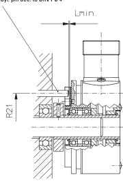
Note: minimum insertion depth 1.5 x  $D_{hollow shaft}$
