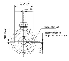
Bracket Type 3 with stator coupling
